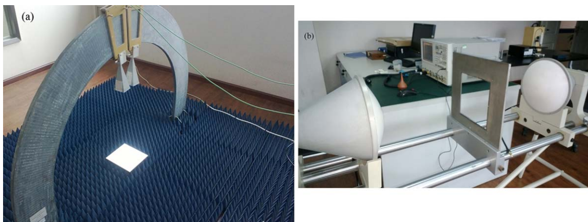
Figure 2. Free-space measurement system: (a) RL measurements and (b) complex permittivity measurements. [Color figure can be viewed in the online issue, which is available at wileyonlinelibrary.com .]
